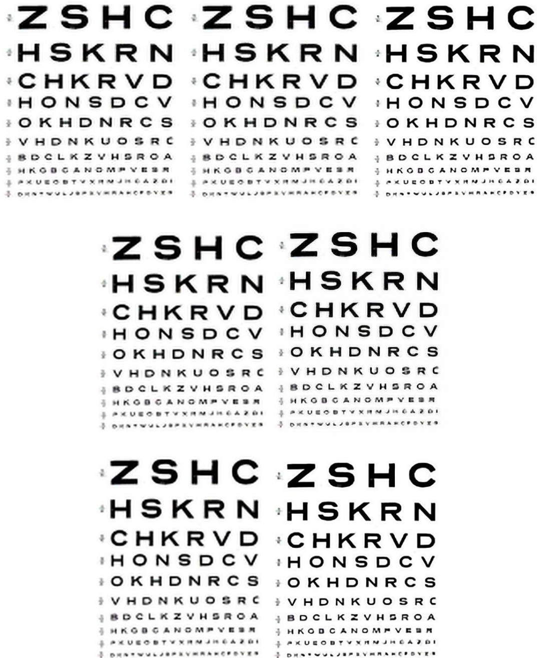
Fig. 5. Comparison of our method with the other methods on text image Eyetest (magnified \times 3 ). Top row: BI (18.961/0.7955), SCSR (20.309/0.8319), SESR (22.713/0.9179); Middle row: ANR (20.005/0.8235), SRCNN (22.1019/0.8836); Bottom row: RAISR (20.143/0.8194) and our method ( 23.126/0.9225 ).
